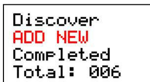
At the start of discovery, all devices will be set to their minimum intensity. As they are discovered, they are set to maximum intensity. This provides a visual cue to the order of short addressing and also highlights any devices that are not operational.
