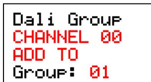
The first option field selects the address of the DALI device to be set. The UP and DOWN keys select:
