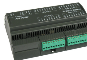
Art-Relay 12-channel mains relay
