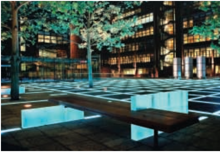
(above and far left) Finsbury Avenue Square features 650 DMX-controlled IP68 LED units, in five different lengths, containing over 100,000 individual LEDs in RGB clusters to offer a full range of colours – all specially developed by Artistic Licence (near left) Regents Place in contrast uses fibre optic cables developed by Philips
