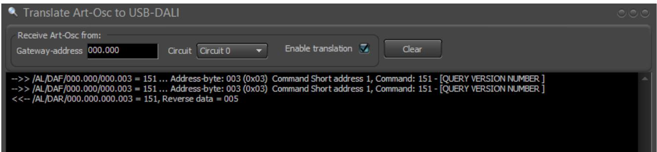
The Gateway-address and circuit define the address of the DALI gateway that the translator will emulate.
